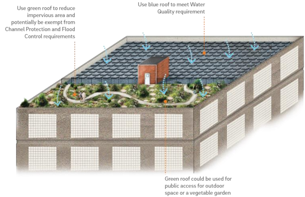
Green and blue roofs can be deployed as part of an integrated stormwater management system (Philadelphia Water Department)
